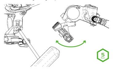
**004\_**Lateral position of the lever can be adjusted using the slotted hole in the direct shifter mount. Further adjustment is possible by swapping the mounting holes on the Dropper lever body. When the desired position is found fully tighten the M5 bolt.
