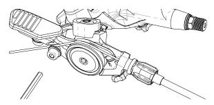
**005\_**Check that the barrel adjuster and reach adjustment screw screwed all the way in, (clockwise turns)
