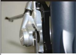
When the brake feels solid, remove the spacing block or pads from the caliper and undo the bleed nipple a 1/4 turn. Use the plastic tyre lever or similar to push the pistons back into the bores (be careful when doing this so as not to damage the pistons, particularly phenolic composite ones) This procedure ensures that any air behind the piston is expelled. Lock bleed nipple off.
