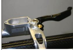
Remove wheel. Position the master cylinder (mc) so the reservoir is horizontal to the ground. Remove the lid and diaphragm from the master cylinder and ensure the lever reach adjust is set with the lever in a 'reasonably' outboard position (not too close to the bar as this affects the feel of the brake) Pads or a similar spacing block should be left inbetween the pistons whilst bleeding.
