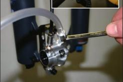
TIP! Make sure fluid is always present in the master cylinder - keep topping up throughout the process
